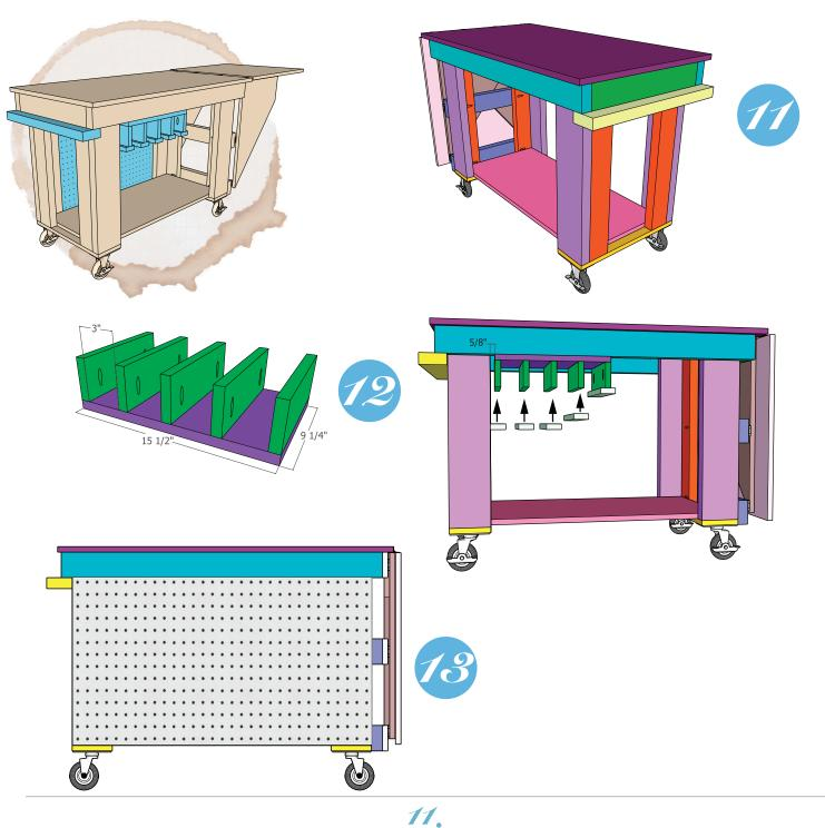
Attach the clamp storage to the opposite end. The 2" x 4" will be flush with the outer edges of the frame and will lay flat up under the frame. Attach with wood glue and 2-1/2 spax screws.
